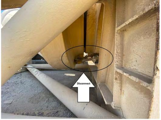
5.5. Lubricate and Grease all the tracks holding jaws of the Hammer and the Pipe Cap slides as shown in below picture.
