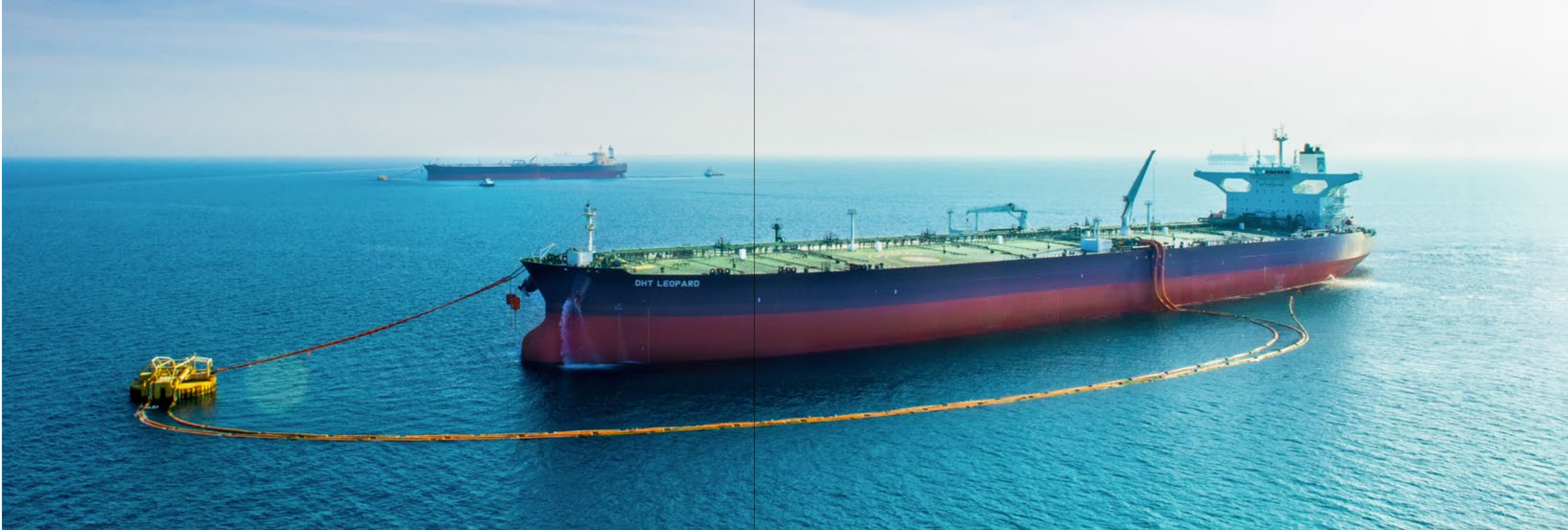
The world calls for energy at the Ju'aymah offshore terminal on the Arabian Gulf, where a supertanker loads crude oil from a single-point mooring.
