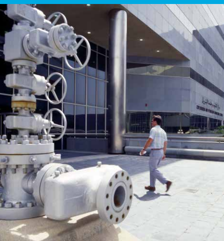
The second wellhead from Dammam Well No. 7, which controlled the well's pressure between 1952 and 1978, stood for years outside the Exploration and Petroleum Engineering Center. Today it's displayed at the King Abdulaziz Center for World Culture.
