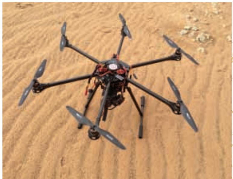
A hexa drone with a high-resolution camera attached to the drone's gimbal, which allows it to move in different directions; and a GPS system on the top (white color) to accurately give the coordinates of each image captured while the drone flies over the flight path.
