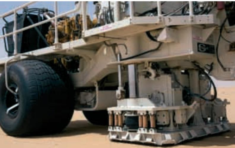
*Left: The vibrator trucks place steel-plated vibration platforms onto the ground to cause seismic waves. Below: GDAD HSE adviser Sadeq Al-Jubran spends much of his time visiting seismic operations across the Kingdom ensuring strict adherence to company HSE policies.*
