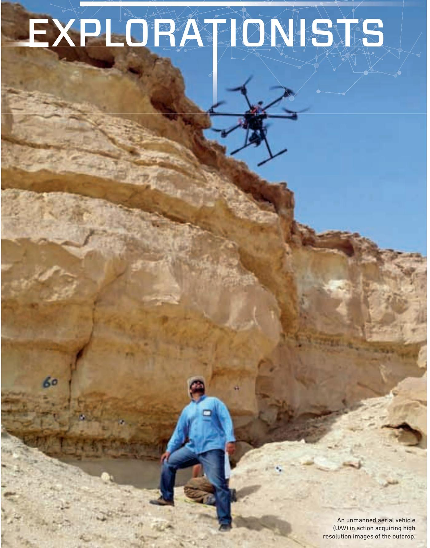
An unmanned aerial vehicle (UAV) in action acquiring high resolution images of the outcrop.
