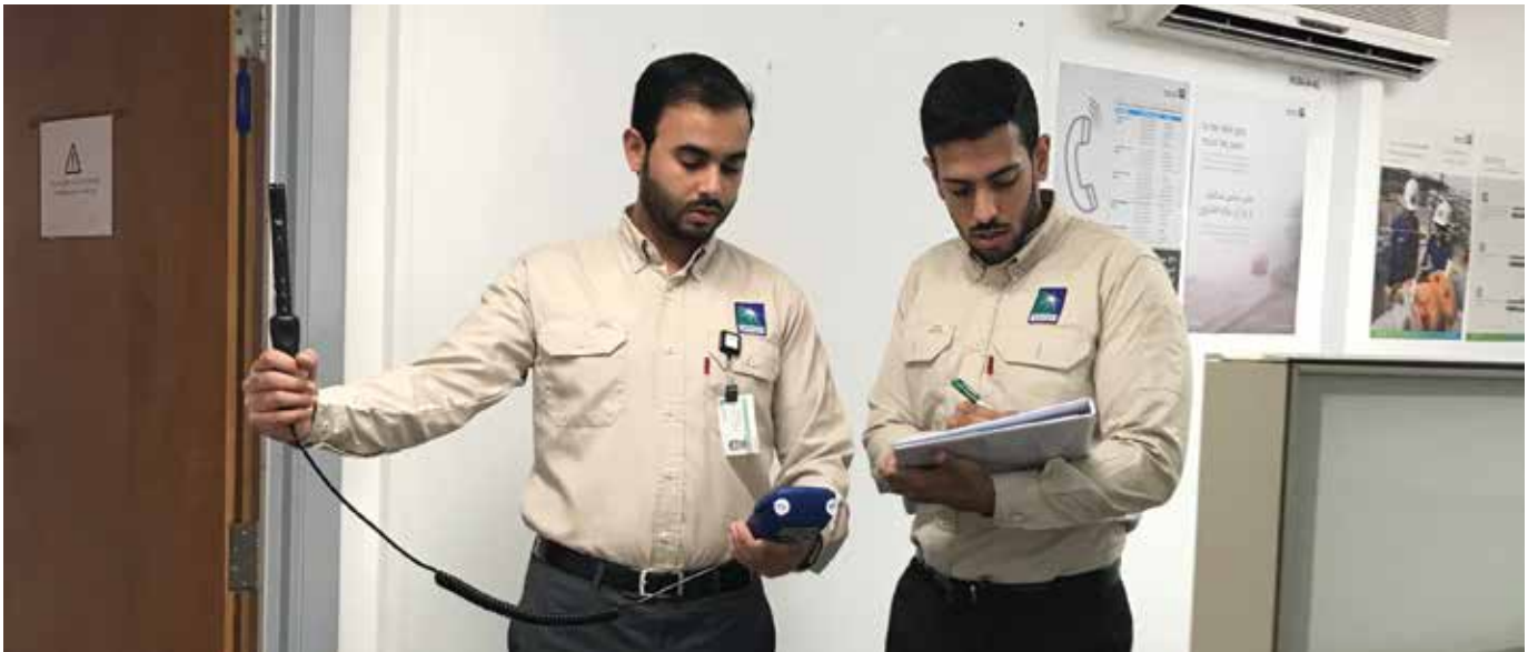
Figure 1. Industrial hygienists take Indoor Air Quality (IAQ) measurements such as relative humidity, temperature, carbon dioxide, carbon monoxide, and other readings to ensure a healthy Saudi Aramco workplace. (Photo Source: Saudi Aramco)
