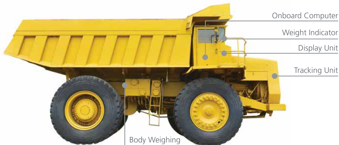
Figure 2: Waste Vehicle Equipped Tracking devices 5 (Photo Source: Shutterstock)
