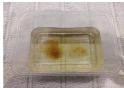
Figure 1. Pure honey has settled on the left, and adulterated honey has dissolved on the right. (Photo Source: Saudi Aramco)
