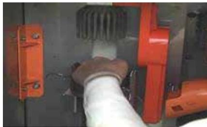
*Figure 2: The feeder from the orange hopper to the juicer.
