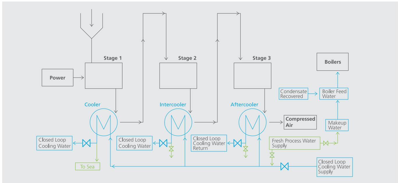
Fig. 1. Process water feeding compressor coolers and then drained to the sea. It was modified to the process in Figure 2.
