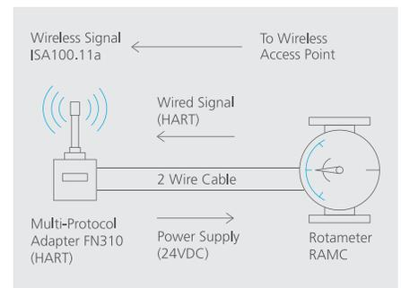
The alarm limits of low and high flow rates have been configured in the DCS to alert operators to take action in case of any deviations in purge quantity. Lower purge rates will result in flare network problems, such as air ingress, corrosion, flameout, while higher flow rates would waste fuel and energy, and also pollute the environment via gas emissions.
