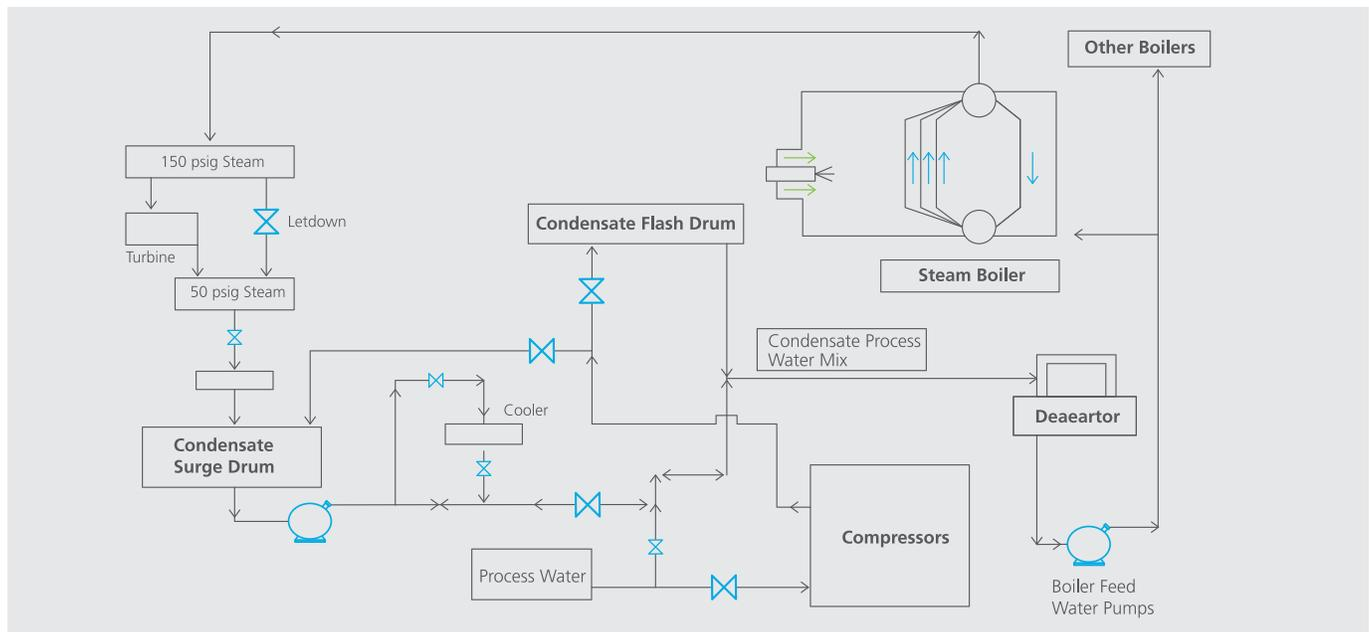
Fig. 2. Innovation Idea implemented: Process water makeup to boilers was diverted to compressor coolers and collected in a condensate flash drum to ultimately use as preheated makeup water. It provided supplement cooling water for use as an independent and redundant cooling source to avoid compressor trips due to cooling deficiencies.
