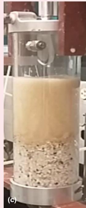
**Fig. 5** The LPLT test using pebble bed for (a) polysweep, (b) polysweep system, and (c) polysweep plus date tree roach root fibers.
