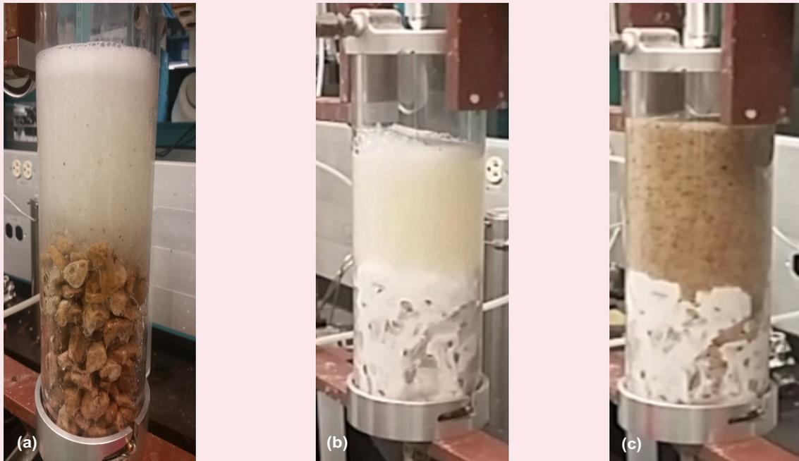
**Fig. 6** Images of the polymer after testing to evaluate its stability under well conditions: (a) at 80 °F with no pressure, (b) at 150 °F and 500 psi, using static pressure, and (c) at 150 °F and 500 psi, after hot rolling.
