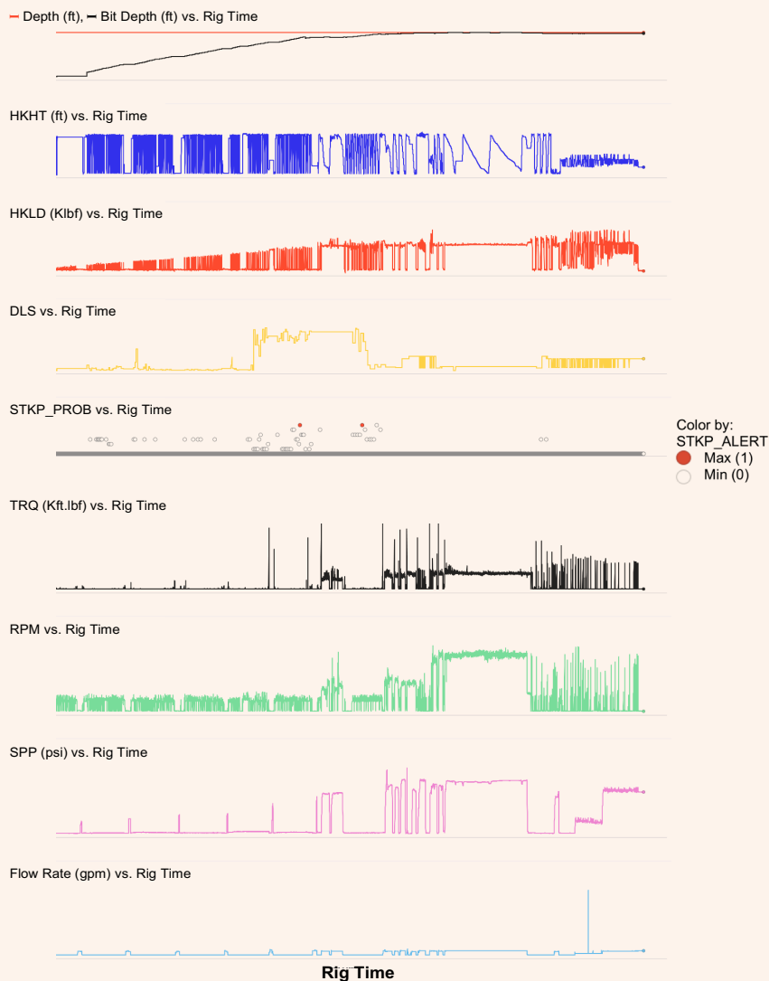
Fig. 6 Two stuck pipe alerts with high probability prior to an incident in Well-A. Highlighted abnormalities included a high DLS value, and an overpull of more than 25 KlbF than the previous HKLD level while RIH.
