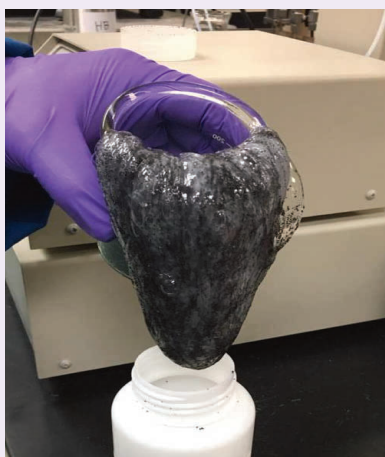
Fig. 5 Proppant laden cross-linked 25 ppt NDFF collected during the main fracturing treatment.
