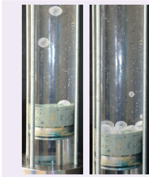
Fig. 10 LCS deployment into the formation orifice.
