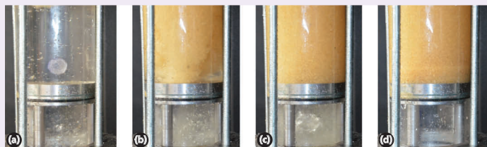
Fig. 9 The faceted LCS deployed to a circular orifice.
